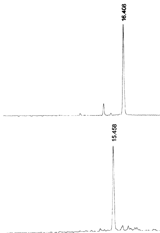
Figure 1. HPLC chromatography at 210 nm of A) the crude chloropeptide 1 and B) the crude thioether cyclic peptide 1 .
